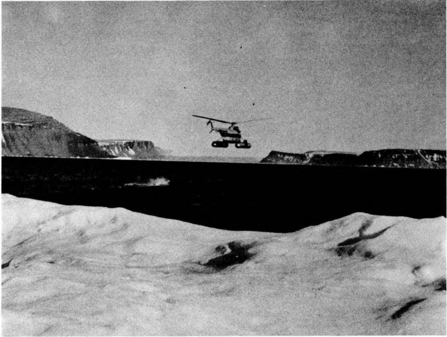
FIG. 3. — Sikorsky S 55 helicopter towing the echo-sounding "fish".
