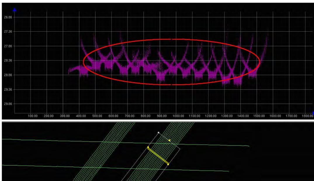
**Figure 6:** The residual systematic errors in sounding swath
