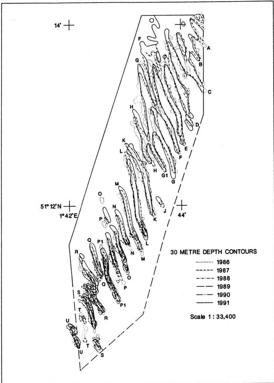
FIG. 4.- Changes to the positions of sandwaves in the Tail of the Falls sandwave field between 1986 and 1991.
