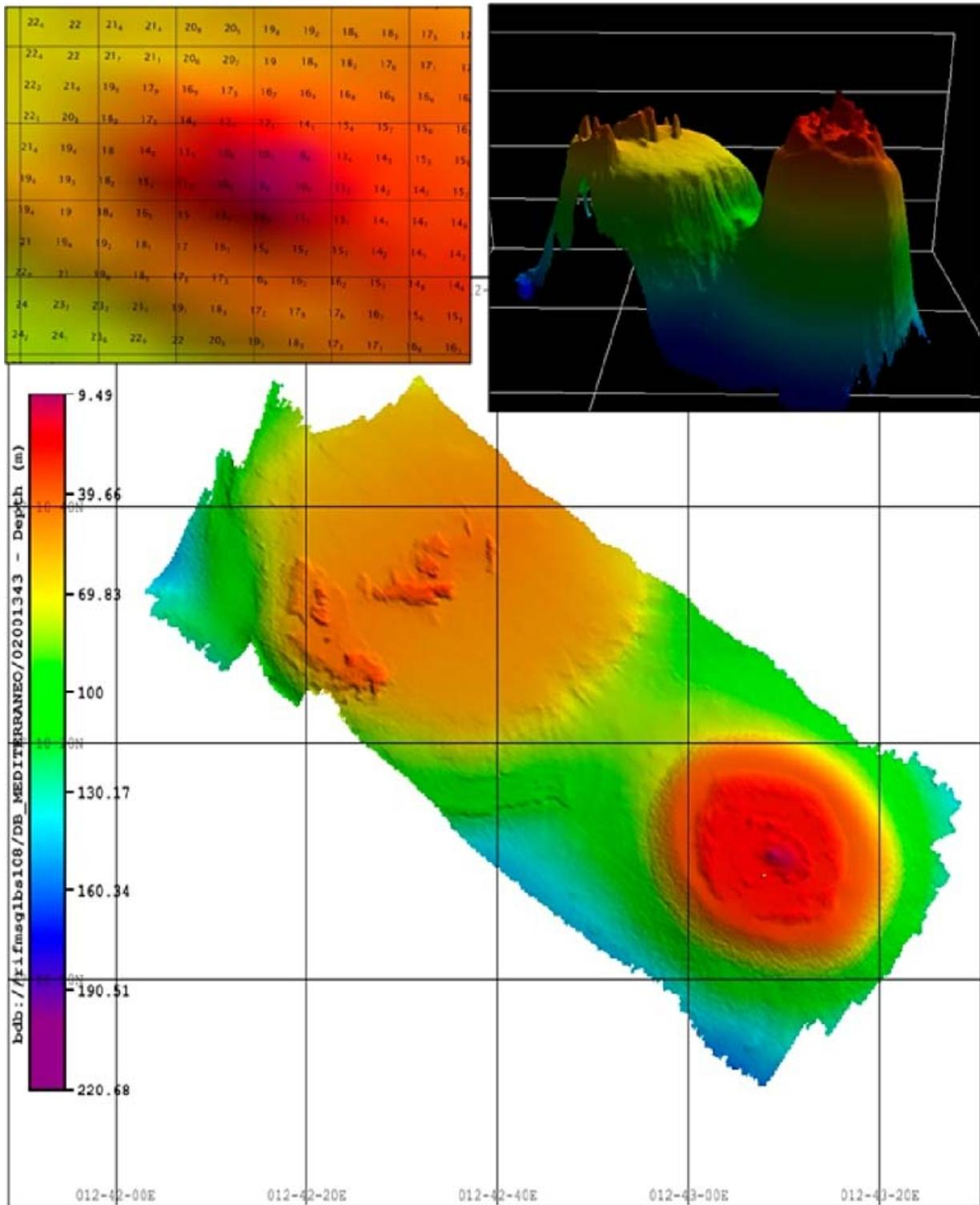
**Figure 7.** Graham Bank bathymetric map 2D model, MB echo sounder survey IIM No. 9091 (2012).
