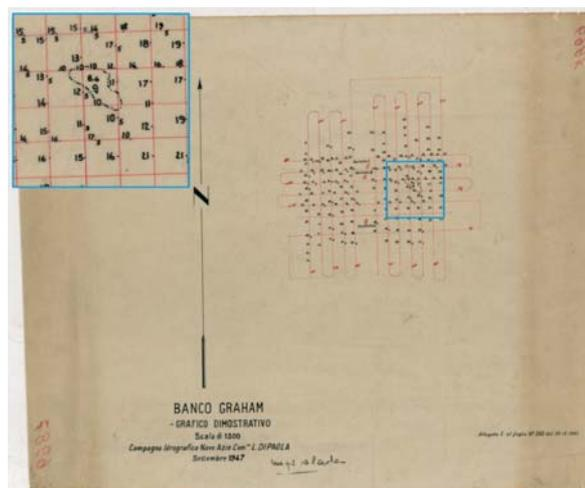
**Figure 4.** Single beam echo sounder hydrographic survey – IIM No 6987 (1947).
