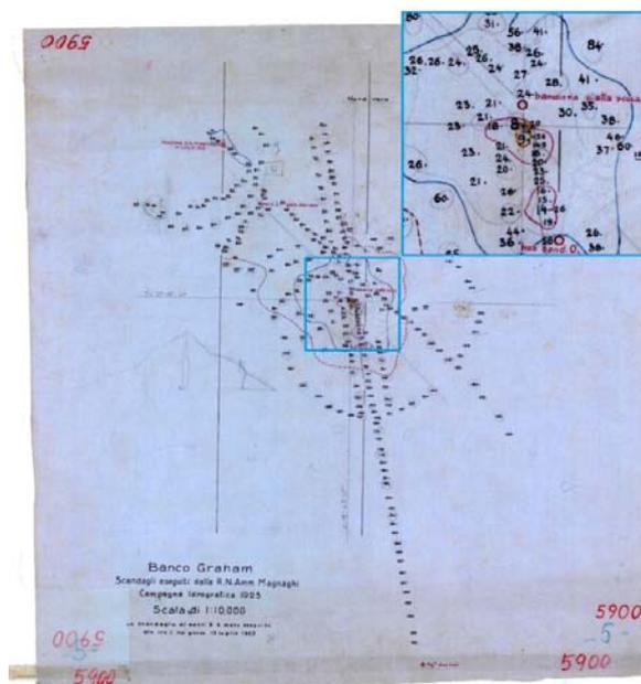
**Figure 3.** Sounding line bathymetric survey - IIM 5900 (1925). Inset shows Graham Bank least depth as 8.0 m.
