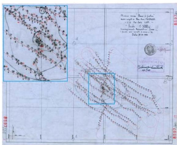
**Figure 6.** Single-beam echo sounder hydrographic survey IIM No 8597-40 (1988).
