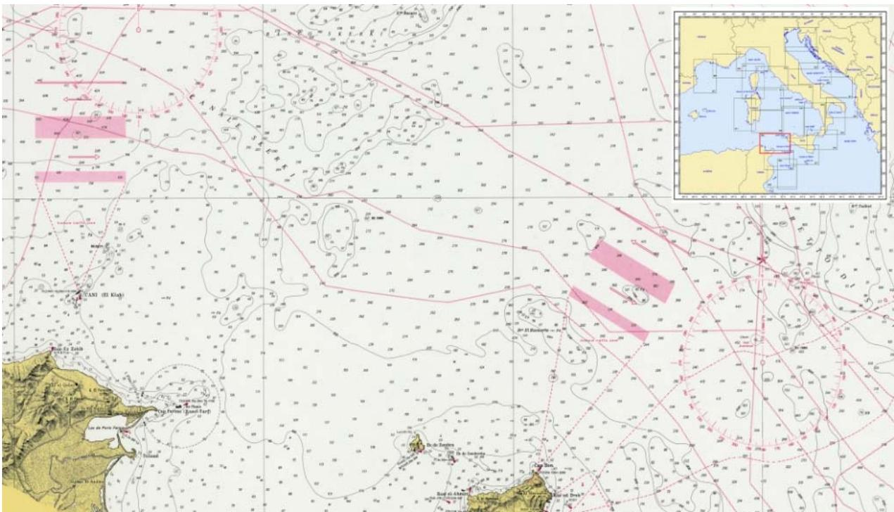
**Figure 10.** Detail of IIM Nautical Paper Chart 948 - Da Bizerte a Ras El Melah Trapani e Pantelleria, 1:250.000 (1998). The inset shows the location. The magenta rectangles show the ships' routing system in the area of the Dog Seamount (left) and the Talbot Shoal (right).
