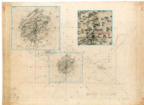
**Figure 2.** Bathymetric survey (lead line) plotting sheet – IIM No 3868 (1890).
