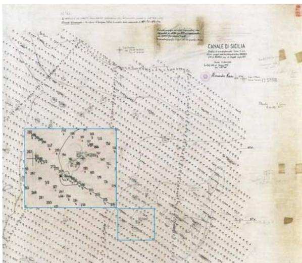
**Figure 5.** Single beam echo sounder hydrographic survey – IIM No 8376 (1977).
