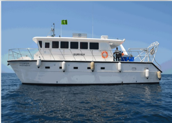
Figure 2. 16m Coastal Hydrographic Survey Launch (HSL) for the GCS
