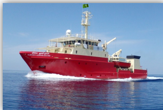
Figure 1. Ocean-going 43.7m Hydrographic Survey Vessel (HSV) for the GCS
