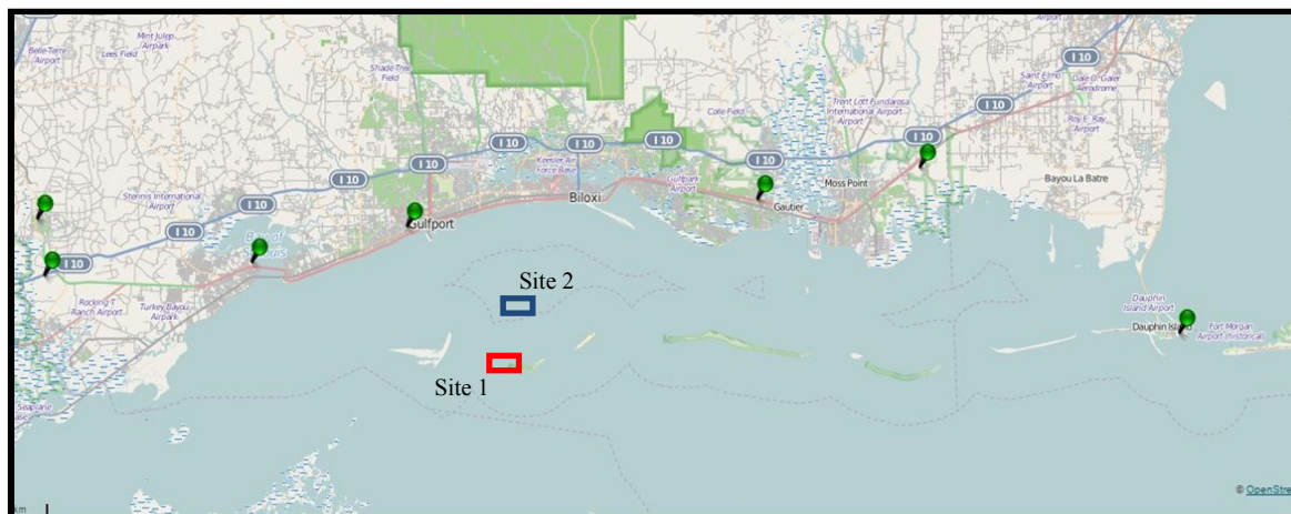
Figure 8. Locations of the reference stations in the GCGC RTN network. The red rectangle is Site 1 and the blue rectangle is Site 2.
