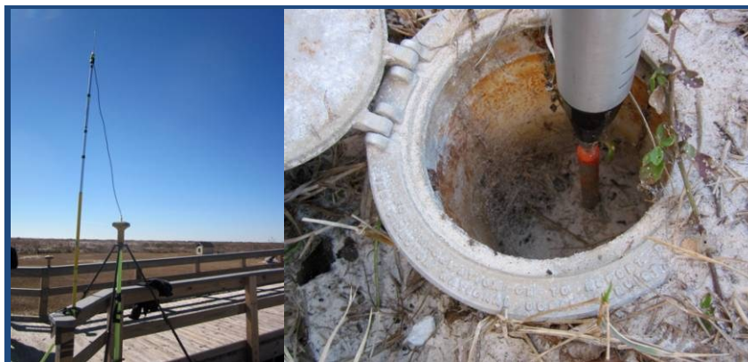
Figure 3. From left to right. GNSS Topcon GR3 with radio link antenna over benchmark on Ship Island. Covered benchmark on Ship Island.
