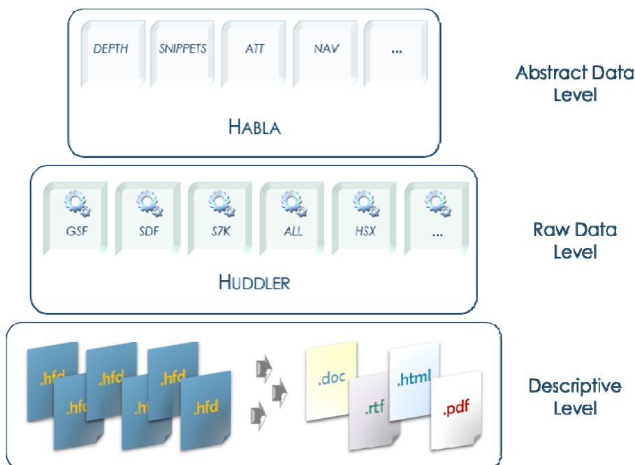
Figure 10 : The three expected levels of users for the HUDDL framework. The basic Descriptive level provides only description services for different file formats, including documentation construction. The Raw Data level provides basic access to particular data formats through automatically generated data drivers. At the Abstract Data level, extra translations provide for conversion of the data into hydrographically understandable information, such as depth or backscatter, without information as to the underlying data format. The HABLA layer is currently under development.
