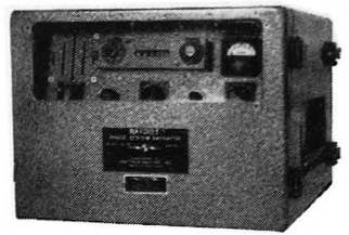
Raydist Range System Navigator, located in moving vessel or aircraft, furnishes accurate, continuous, and automatic reading of range from Raydist Buoy.
