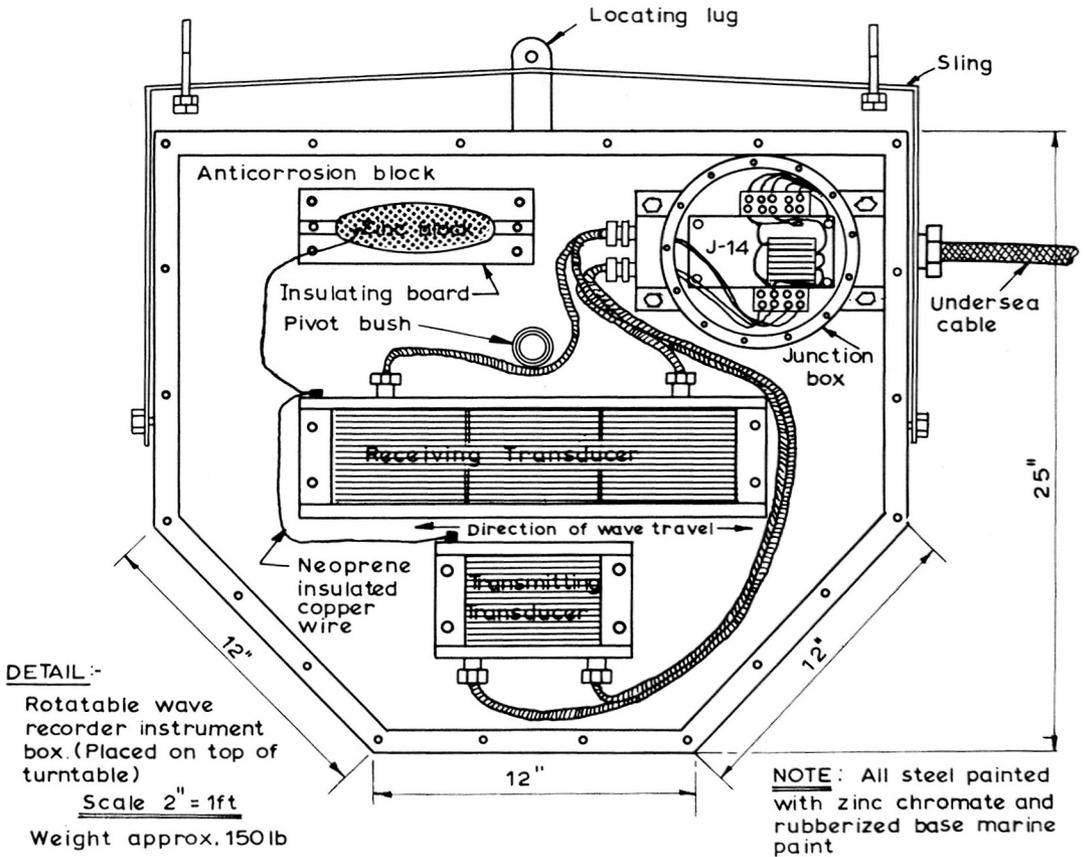
FIG. 5. — Details of the transducer assembly & housing as mounted on top of the stand (Figs. 3 & 4).
