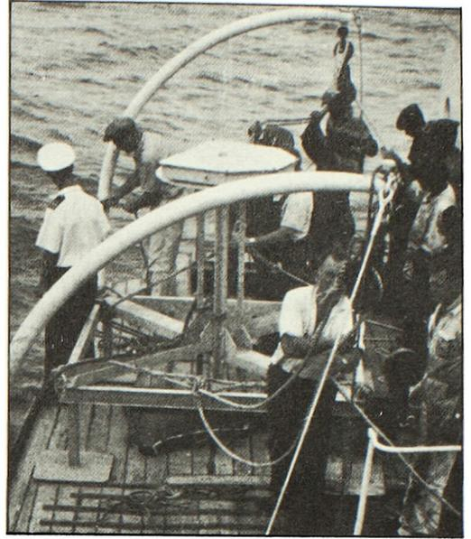
FIG. 4. — The stand carrying the transducer assembly, with cable connected, just before it was lowered from davits into 76 ft of water.
