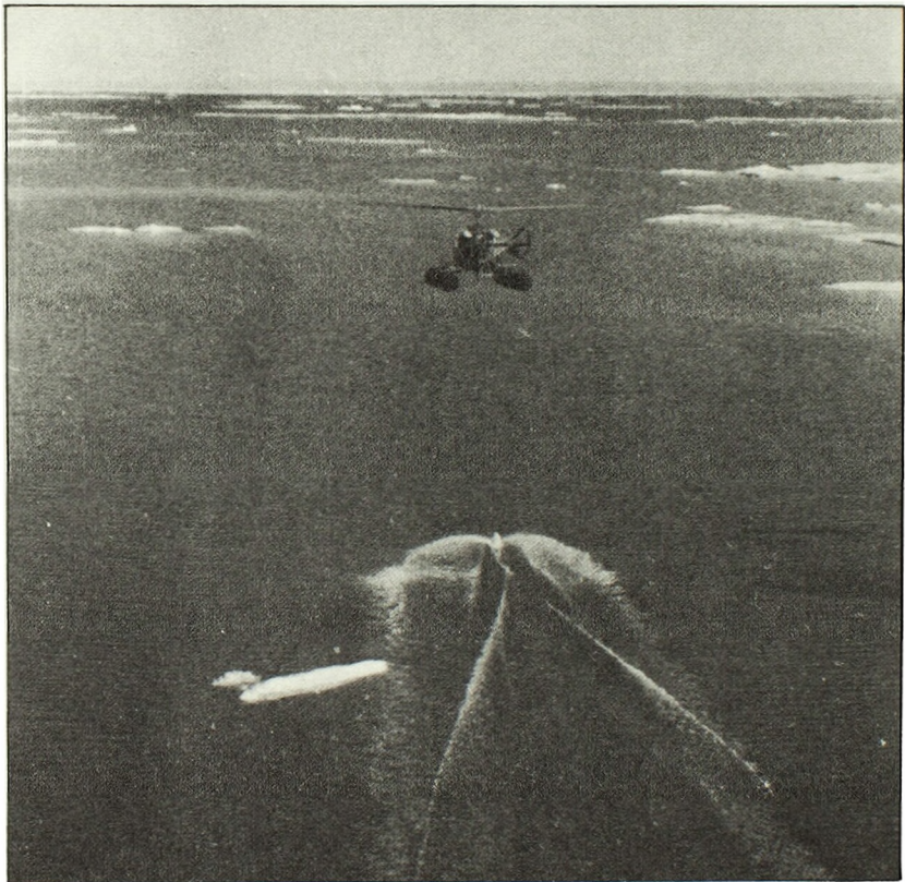
FIG. 4. — A Bell 47 G2A helicopter towing. The sea state here is ideal; enough ripple for the pilot to judge his height (which becomes difficult over calm water) yet not so rough as to cause heavy drag on the Float. The Fish can easily be manoeuvred through open ice like this.
