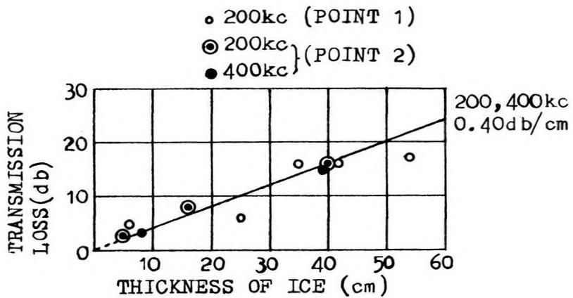
FIG. 14. — Transmission loss in ice from Lake Haruna.
