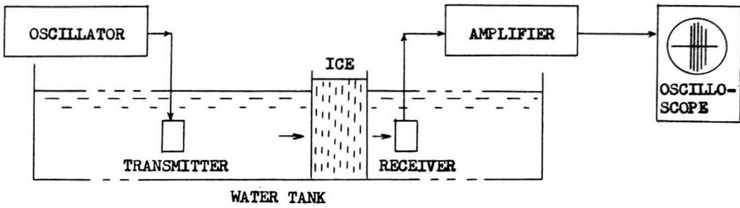
FIG. 11. — Method of measurement of transmission loss of ultrasonic waves in ice.
