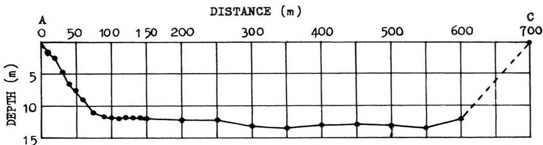
FIG. 10. — Transverse section of Lake Haruna established from the echo traces obtained the surface of the ice.
