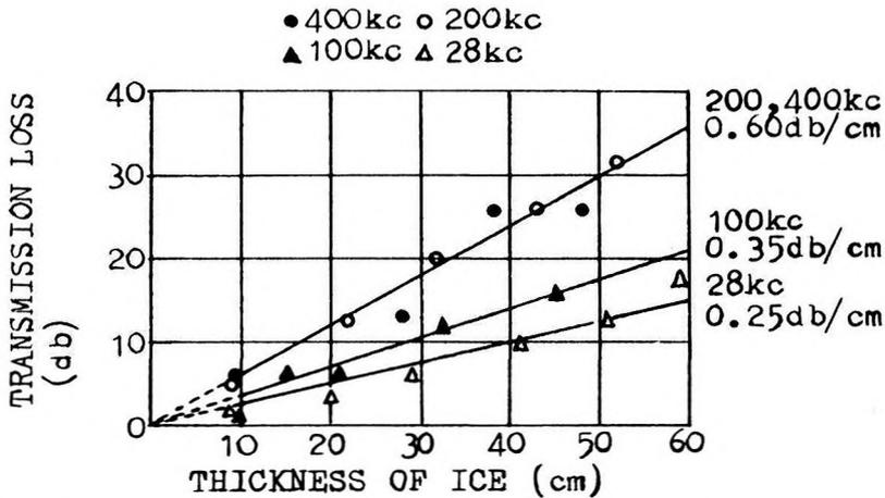
FIG. 12. — Transmission loss in artificial ice such as can be found on the market.
