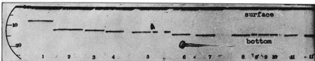
FIG. 9. — Echo trace of lake bottom when sounded from the surface of the ice (400 kc/s; thickness of ice : 25 cm).
