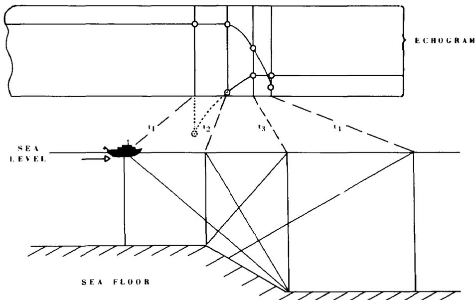
FIG. 3. — Schematic diagram showing the relationship of the seafloor profile and the resulting echogram.
