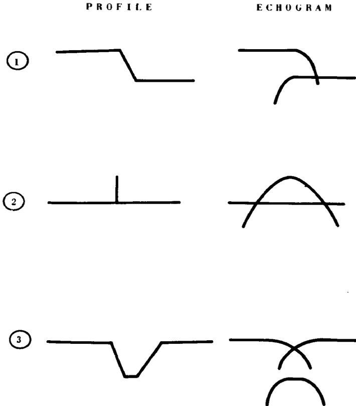
FIG. 4. — Qualitative comparison of profiles of seafloor profile and the echograms.
