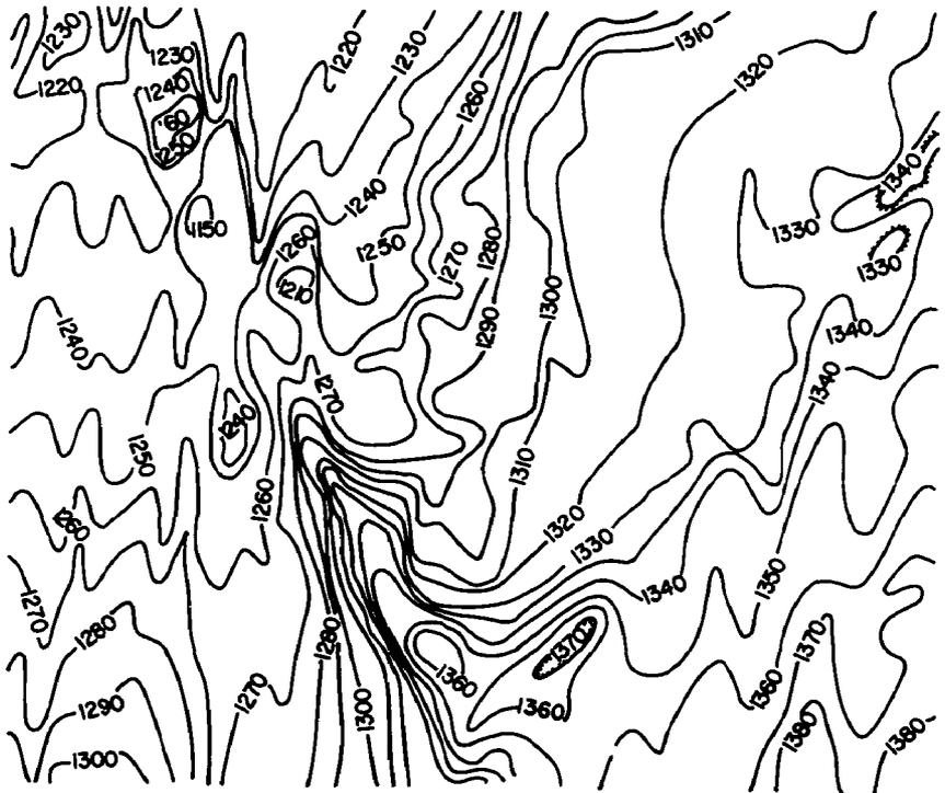
FIG. 6. — Contours based on first arrival sounding echoes and without any navigation corrections.
