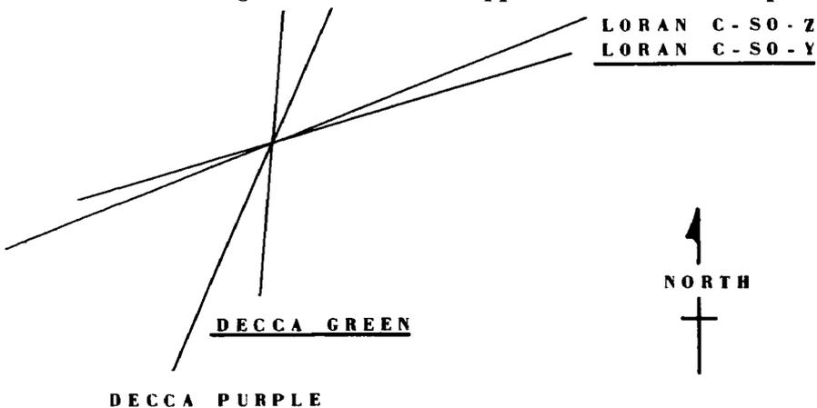
FIG. 1. — The relative angles of intersection of the available navigation lines.
