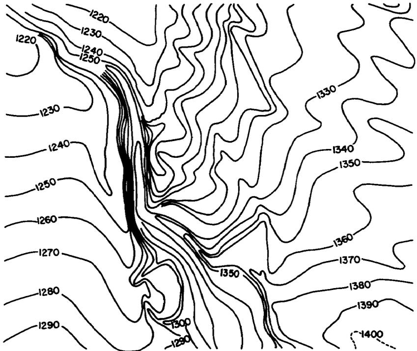
FIG. 7. — Same area as Fig. 6, contoured using corrected navigation and interpreted depths.
