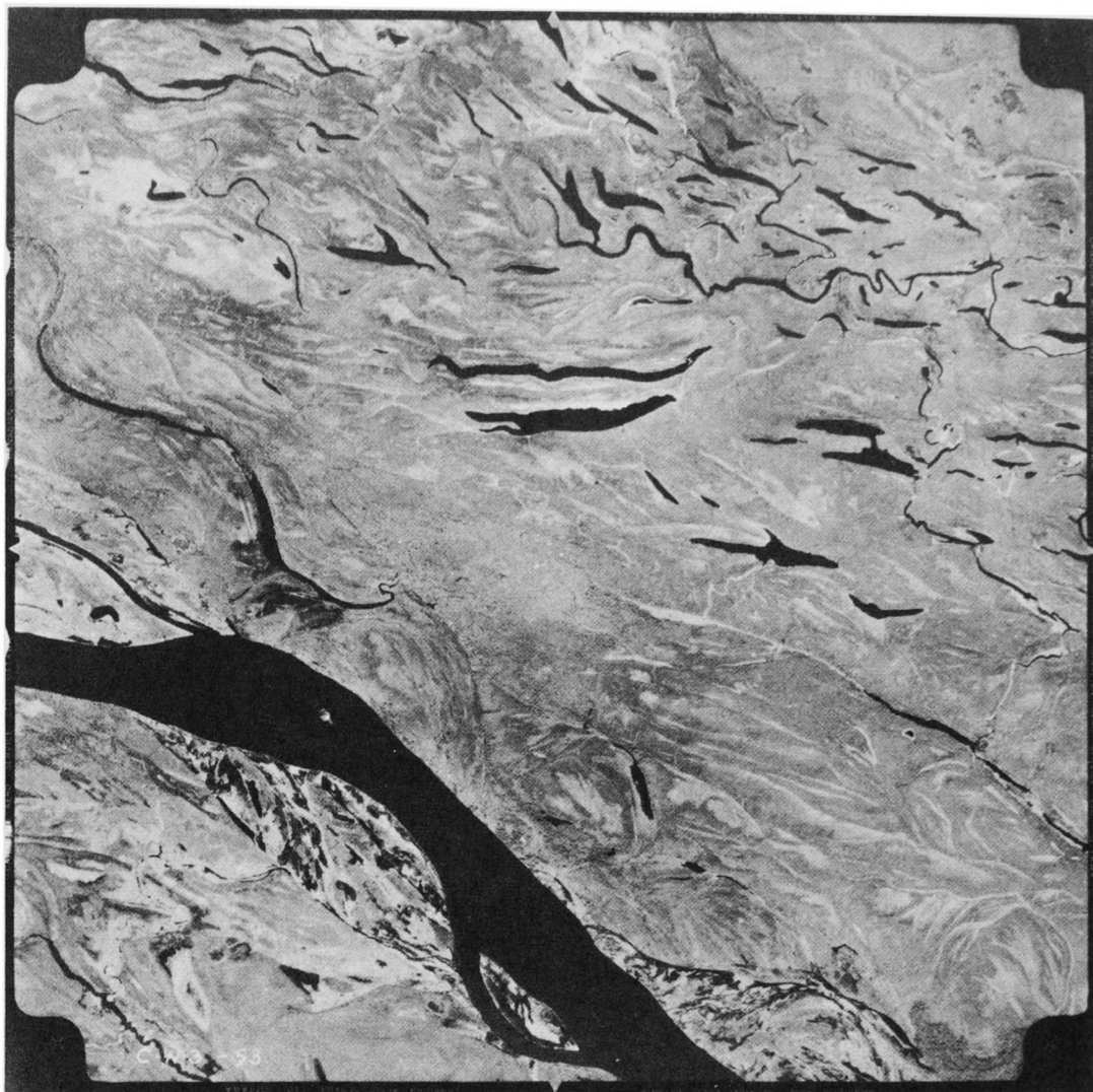
FIG. 20. — Aerial photograph taken in Nigeria with a Wild RC-9 camera equipped with super-infragon lens and using infra-red film.
