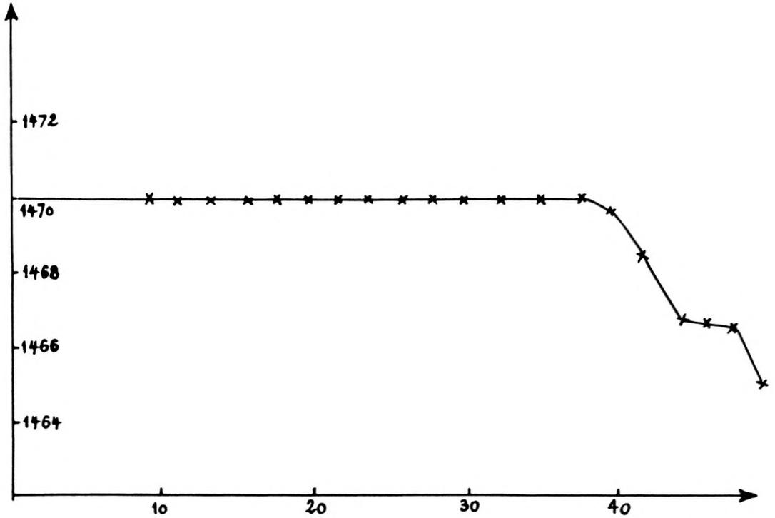
FIG. 4. — Towing tank trials. Sound velocity versus towing speed.
