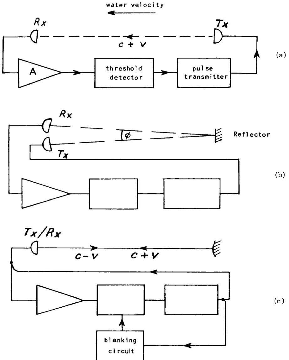
FIG. 1. — Sing-around velocity meter systems :
