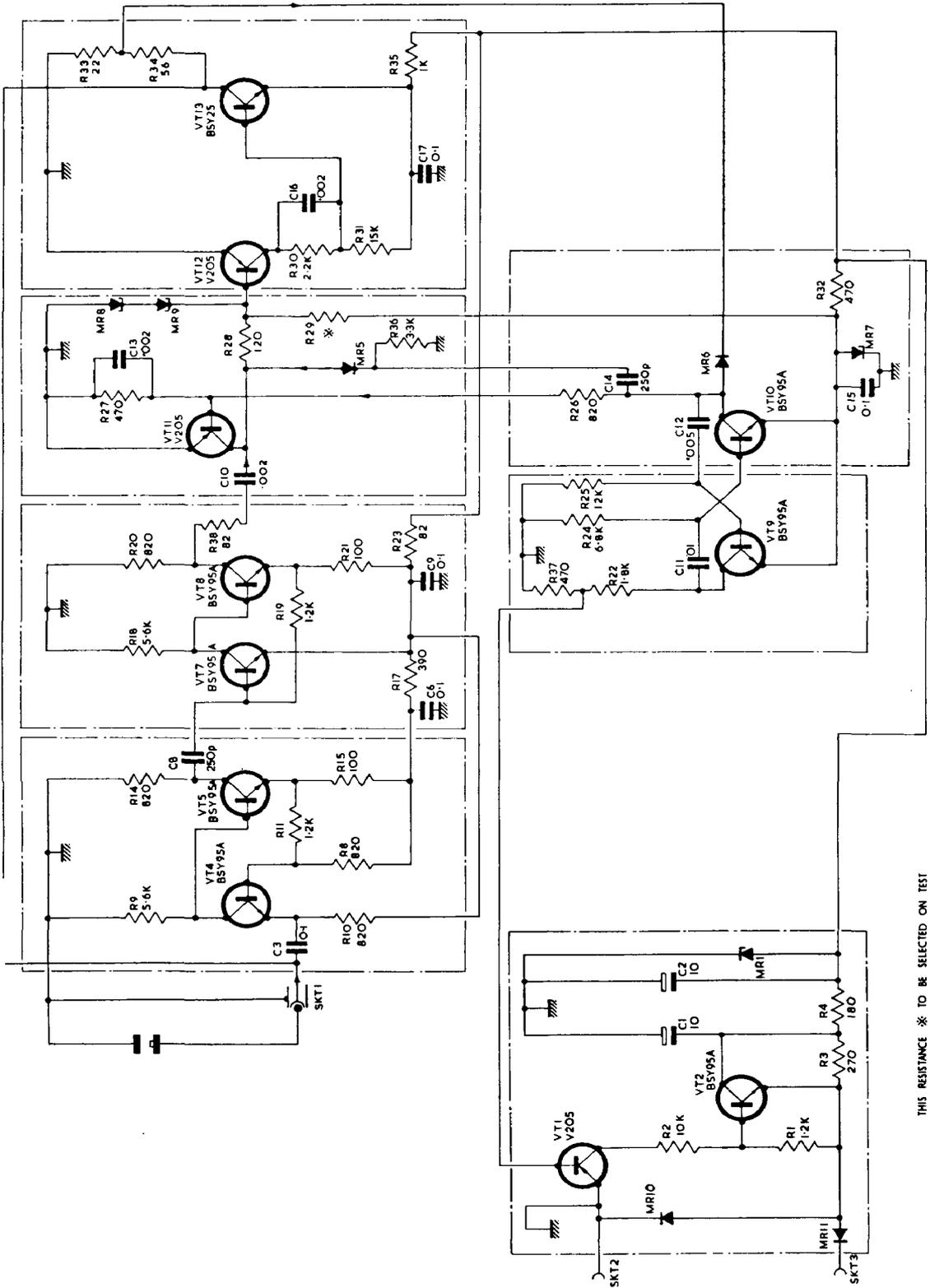
Fig. 3. — Circuit diagram of Sound Velocity Meter, type MO31.
