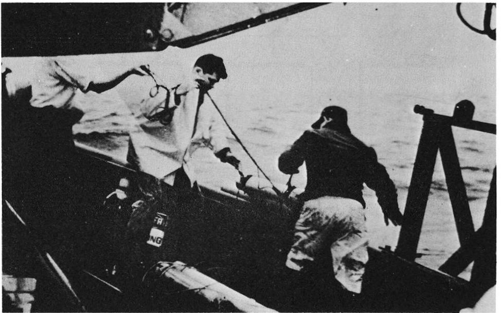
FIG. 4. — Putting the transponder over the side.
