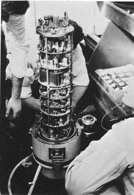
FIG. 1. — The probe's electronic unit.
