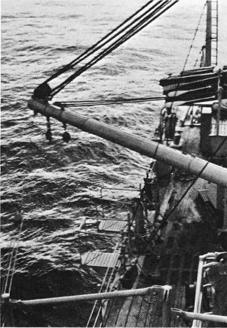
FIG. 5. — The *Origny's* starboard deck, with derrick in working position.
