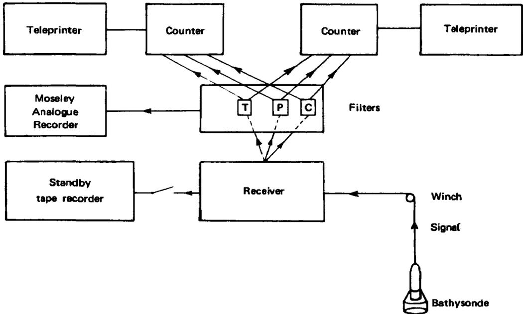
FIG. 9. — Flow diagram of the recording system used during the Medoc 69 Project.
