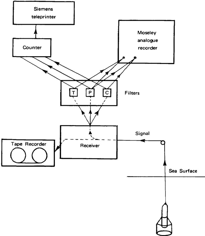
FIG. 4. — Flow diagram of the measurement processes.
