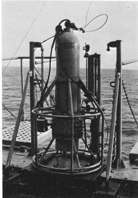
FIG. 2. — The Howaldt Bathysonde mounted on its cradle ready for use.
