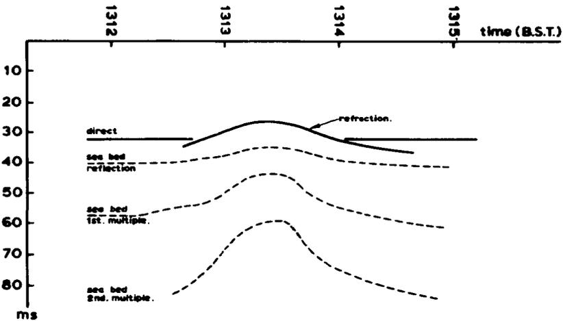
FIG. 2. — Sketch of sparker time-section showing refracted arrival, obtained off the Gower Coast, Glamorgan.
