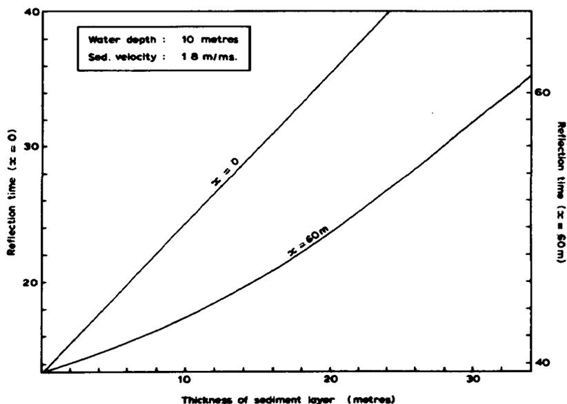
FIG. 3. — Effect of source-hydrophone separation on sub-bottom reflection times.
