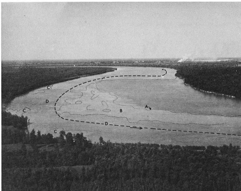
FIG. 15. — Low-angle, oblique, aerial photograph showing distribution of water turbulence during flood stage, Thomas Point, Mississippi River. The letter symbols indicate the same zones as shown on figure 14. Dashed line indicates the deep-water channel.
