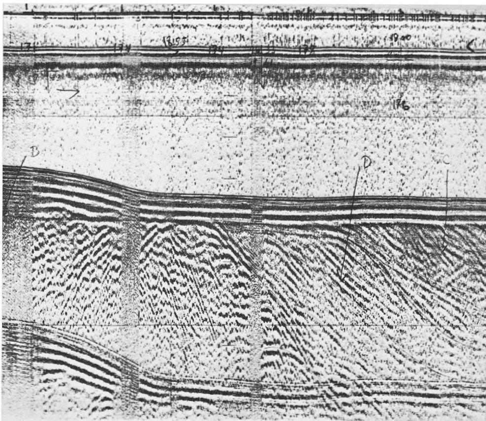
FIG. 10. — Effect of filtering on a 3 000 J Sparker record. The 200-800 Hz filters on the left are too high to obtain a good record. The operator then tried 80-800 Hz which gave him a better result (100 ms between scale lines).
