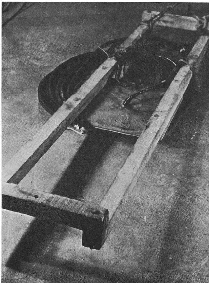
FIG. 2. — The *Boomer 300 J* on its fish.
