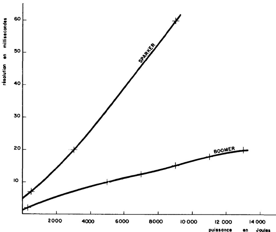
Fig. 11. A curve showing resolution as a function of electric power for the *Boomer* and the *Sparker*.
