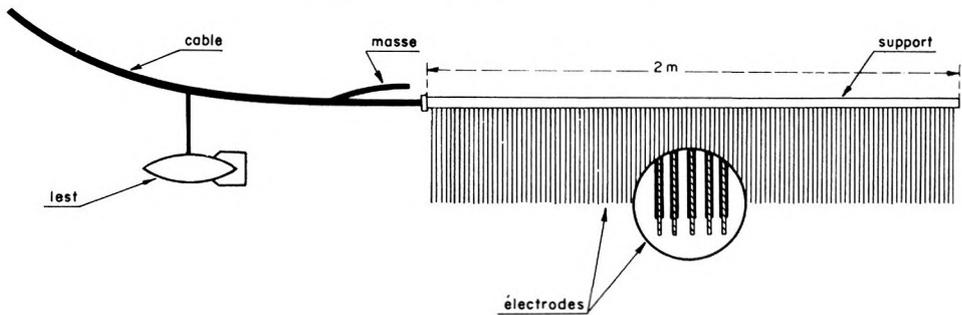
FIG. 5. — Sketch of an "Etinceleur". This instrument works at 1 to 5 J per electrode on an electronic circuit such as is shown in figure 1. The gain in resolution is due to the fact that the bubble is reduced in size, having been split into a large number of small bubbles.
