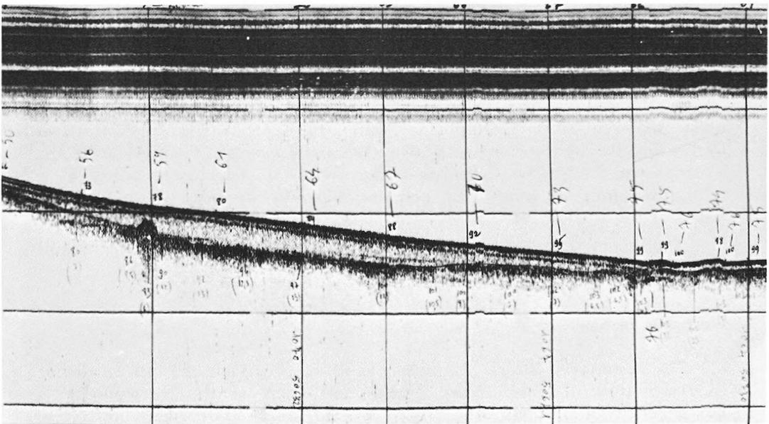
FIG. 6. — Profile from a sediment probe. Effect of source depth on resolution. The fish is being trailed at too great a depth. It is seen that the signal is split by reflection from the surface, and this is prejudicial to the resolution (vertical scale : 40 ms between the horizontal scale lines; horizontal scale : 900 m between vertical marks).
