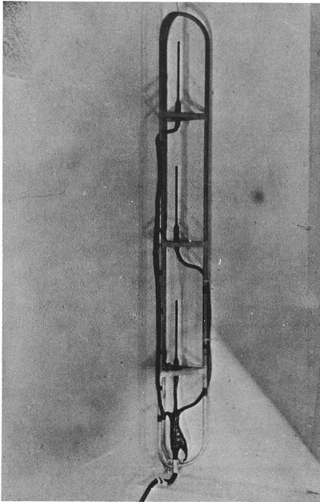
FIG. 4. — The *Sparker* 9 000 J manufactured by E.G. & G. This instrument works at 1 000 to 5 000 J per electrode. It is plugged into an electronic circuit of the type shown in figure 1.
