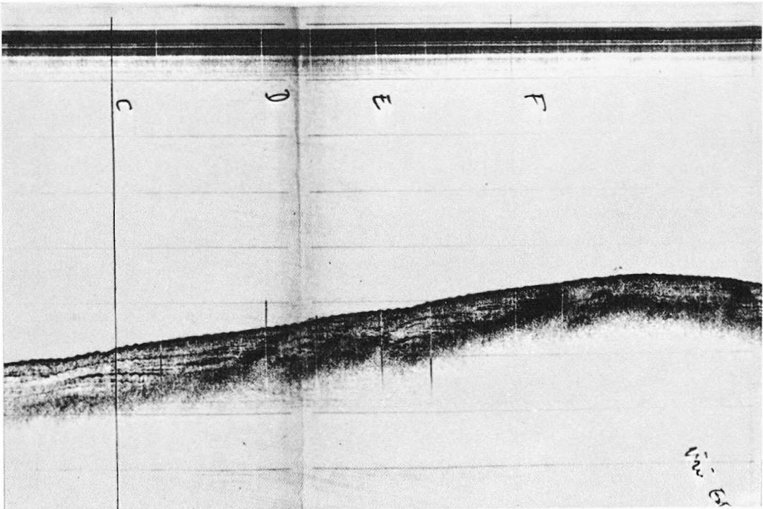
FIG. 9. — Profile from the "Mud Penetrator" sediment probe. At a 12 kHz frequency a resolution of better than 150 ms is achieved (10 ms between scale lines).
