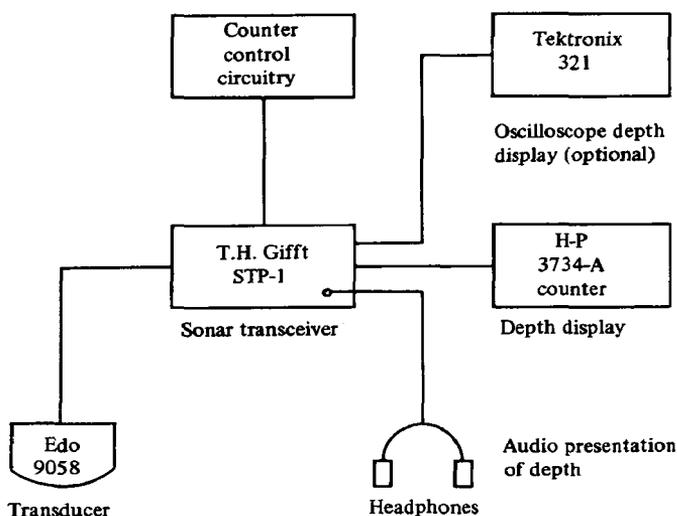
FIG. 1. — Sounding System Block Diagram.
