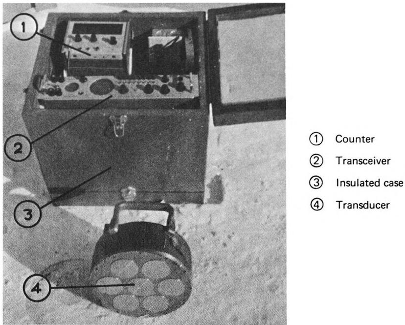
FIG. 2. — Equipment and carrying case.
