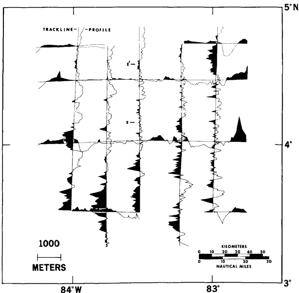
FIG. 2. — Bathymetric profiles from southern part of survey area presented along tracklines (see figure 1). The blackened portions of the profiles represent depths shallower than the average depth along each trackline segment. Vertical exaggeration for each profile is about 20/1. Relief of the microtopography is given by the 1 000-metre scale. The fathogram record between E and E' is shown in plate 2.
