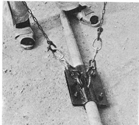
FIG. 3. — The device made up of lengths of iron piping.
