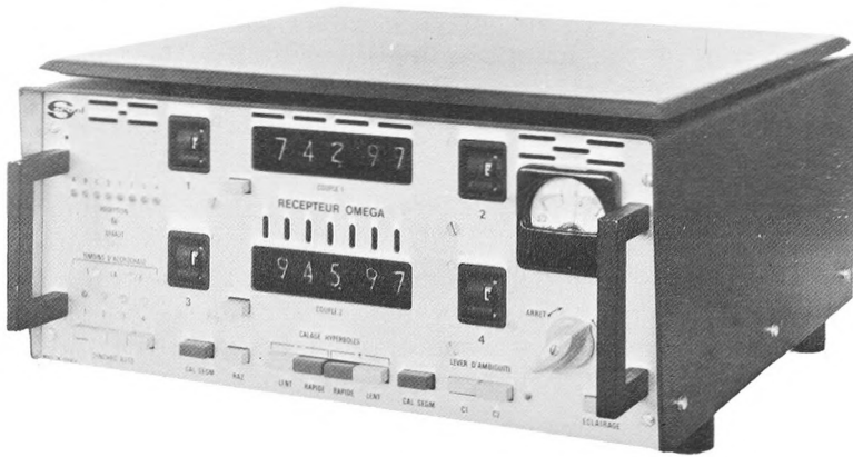
Fig. 1. — Dual-frequency receiver, model RR.FX.2.A, with automatic lane identification, as accepted by the French Navy.
