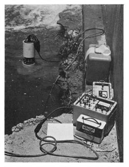
**HYDROLAB SYSTEM,** a modern and reliable in-situ apparatus consisting of a control unit, cable and underwater sonde with sensors to measure various parameters including Temperature, Depth, Conductivity, Dissolved Oxygen, pH, etc. A field recorder provides a graphic record.
