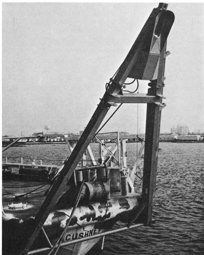
FIG. 11. — Support ship A-frame and billboard.
