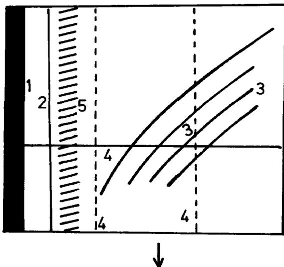
FIG. 2. — A side scan record. Explanations are given in the text. Note, however, that the geologic features (3) are simplified; (4) indicates the two scale lines and a time mark; and (5) the secondary lobe of the transducer.
