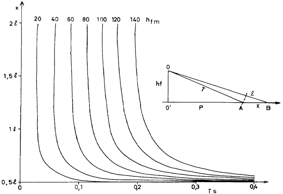
FIG. 5. — Effect of the pulse length on resolution.  $l$  is the path corresponding to the pulse length, and  $X$  the resulting loss of resolution. Entering  $T$ , from the time read on the recorder, the resulting curves will indicate the loss of resolution in terms of pulse length and the transducer height above the bottom. (Figure taken from CHOLET *et al.*)
