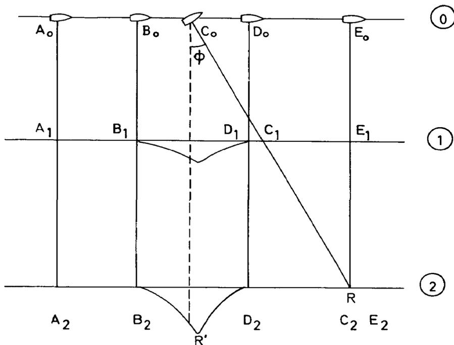
FIG. 9. Effect of yawing of the fish. (after CHOLET *et al.*)
