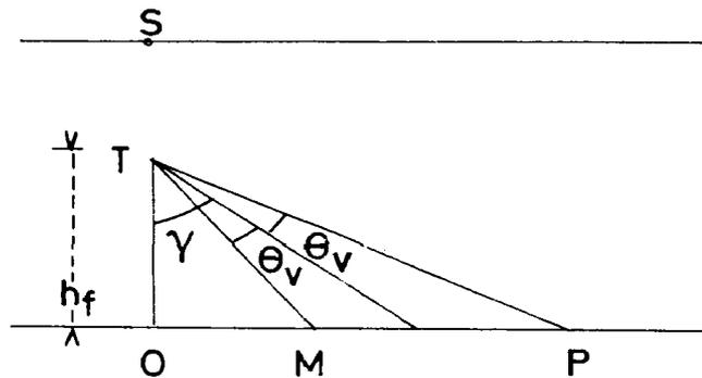
FIG. 3. — Vertical section, showing the shadow zone OM, and the scanned area MP. S indicates the ship.
