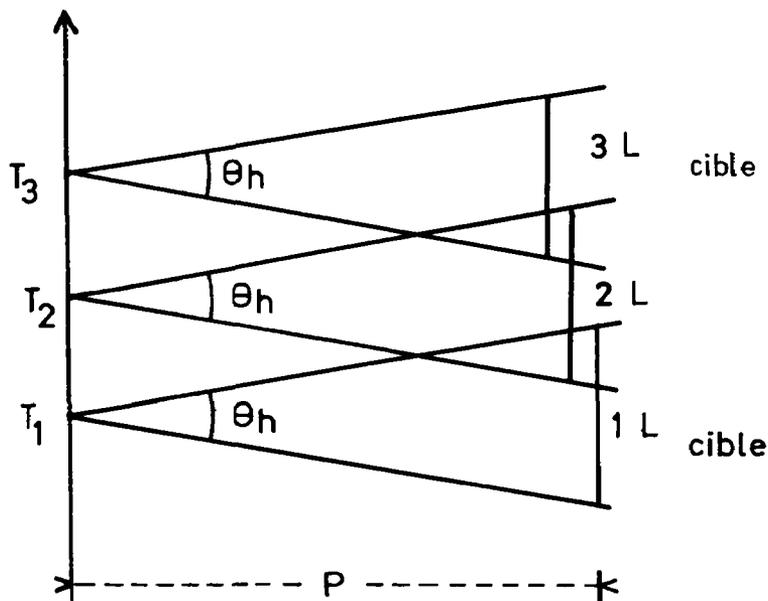
FIG. 6. — Successive positions of the surfaces covered by a transducer moving from position 1 through to position 3.
