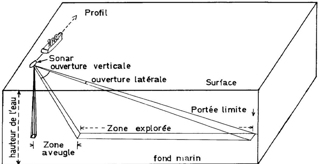
FIG. 1. — Principle of a side scan sonar.
