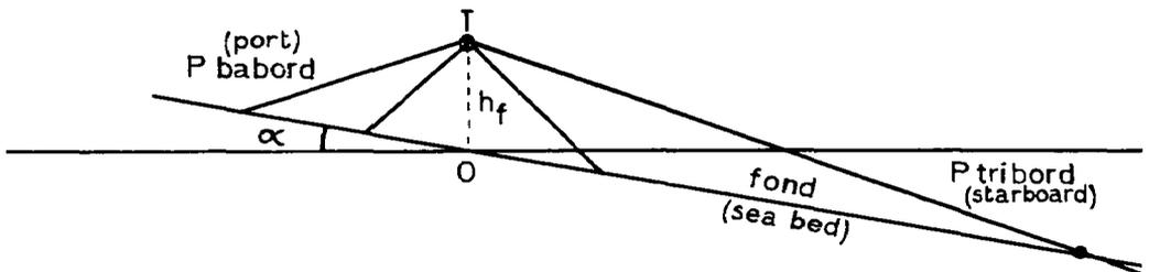
FIG. 8. — Effect of the inclination of the bottom on range.
