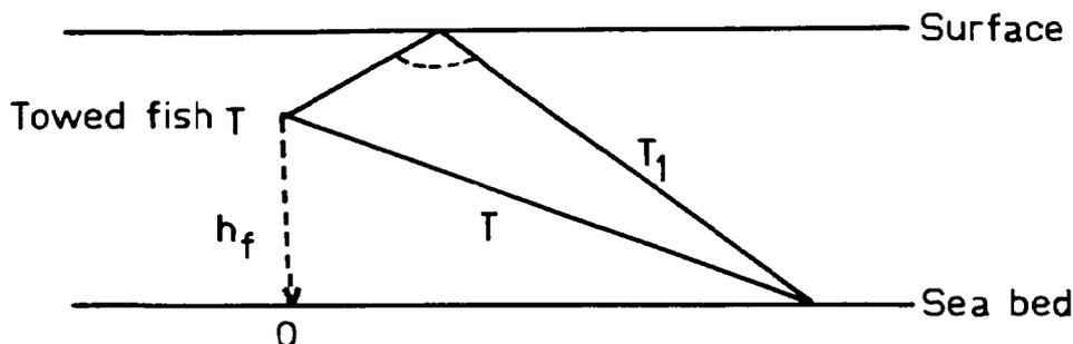
FIG. 11. — Diagram showing how interferences are formed between a normal path T and a path T<sub>1</sub> that has been reflected once on the water surface.
