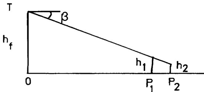
FIG. 4. — Effect of the height of two targets on the resolution. In this example  $h_2 = P_2 \tan \beta$ .
