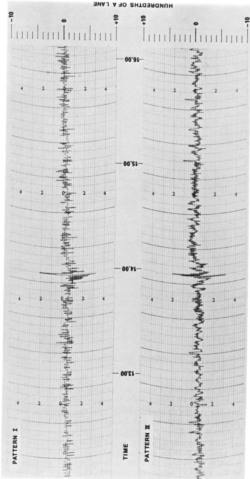
FIG. 2. — Pattern fluctuations caused by a large vessel passing close to the Sheerness monitor station at 14.00 on 21 March 1971.
