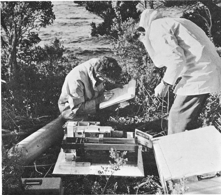
FIG. 4. — Tide gauge installed far from reach of waves. Note gas bottle (left), batteries, bubbler controls, paper punch (centre), insulating lid (right).
