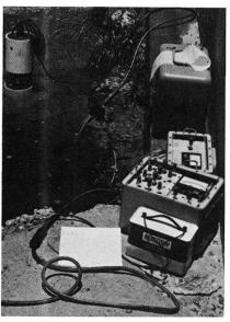
HYDROLAB SYSTEM, a modern and reliable in-situ measuring and monitoring system consisting of a control unit, cable and underwater sonde with sensors to measure various parameters including Temperature, Depth, Conductivity, Dissolved Oxygen, pH, Specific lon, etc. Accessory recorders and data loggers are available.
