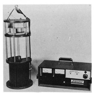
REMOTE CURRENT METER, uses a special Savonius rotor and coupled compass to provide accurate measurements of water speed and direction. Special design features make this the most reliable unit available. Accessory recorders and data loggers can be provided.
