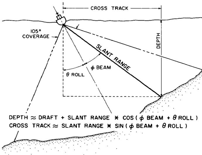
FIG. 2. — Simplified diagram of beam geometry.
