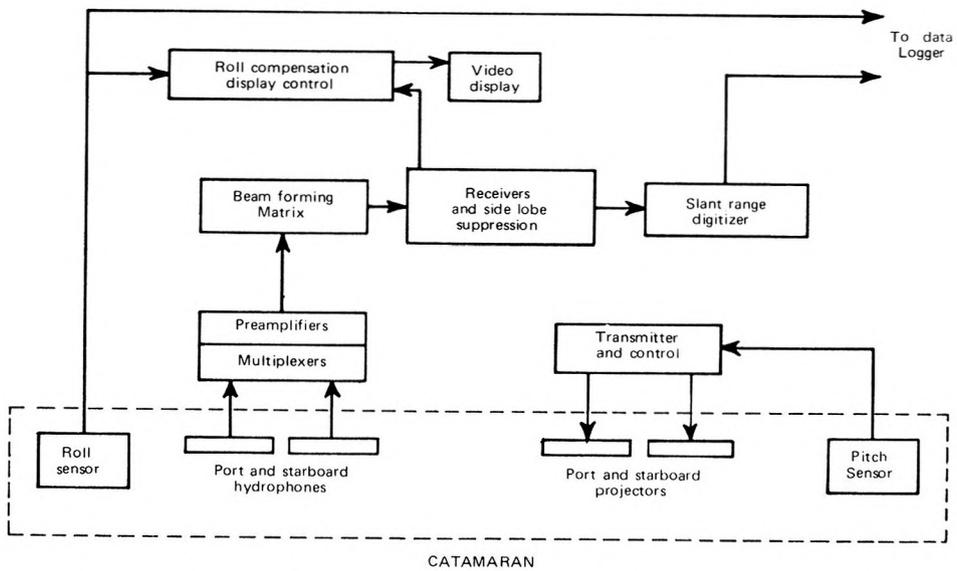
FIG. 7. — Simplified block diagram of Bos'un multibeam signal processing.
