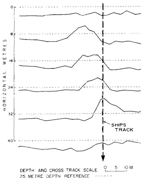
FIG. 10. — Depth profiles of submerged wreck obtained from BO'SUN data.
