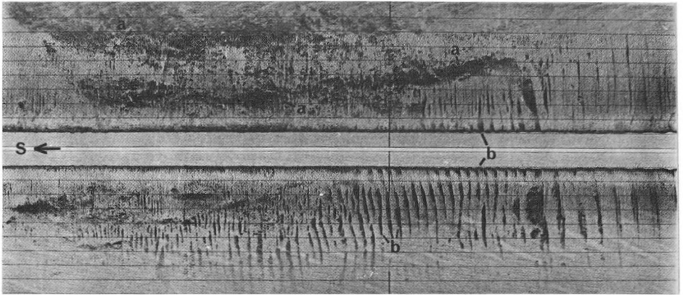
FIG. 22. — Dark reflectors are here produced by material (a) as well as topography (b) Large sand waves break up in the turbulent flow produced by the rough bedrock surface
