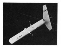
Current speed, current direction, time and temperature are recorded at preselected intervals on a magnetic tape cassette. Flexible programming of data format allows for deployment under a variety of survey conditions.
