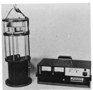
HYDROLAB SYSTEM, a modern and reliable in-situ measuring and monitoring system consisting of a control unit, cable and underwater sonde with sensors to measure various parameters including Temperature, Depth, Conductivity, Dissolved Oxygen, pH, Specific Ion, etc. Accessory recorders and data loggers are available.
