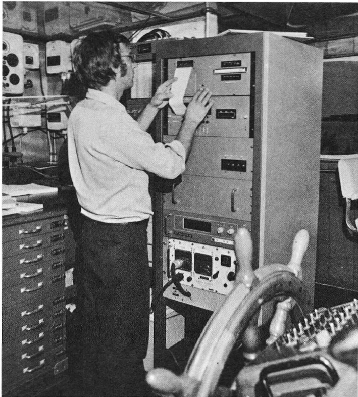
FIG. 3. — INDAPS data logger installed on a survey vessel.
