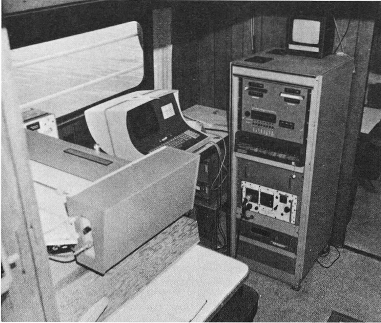
FIG. 2. — INDAPS logger/processor installed on a survey vessel.
