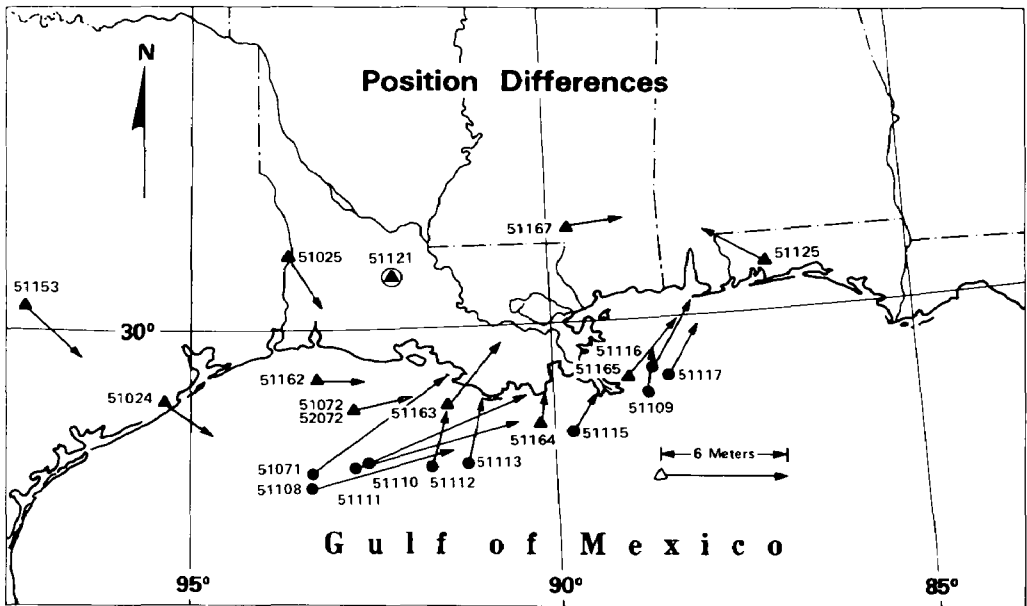
FIG. 4. . . Position Differences. This illustration is the same as fig. 3 except for the addition of offshore Doppler stations which had unadjusted NAD 1927 Datum positions established by non-NGS surveys. The symbol (•) indicates these stations.
