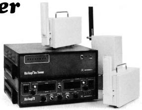
The Mini-Ranger III™ position determining system can tell you exactly where you are — in boats, dredges, helicopters, instrument recording trucks, or other survey vehicles — at ranges from 100 feet to 100 nautical miles. And with probable range error of less than 3 meters.
