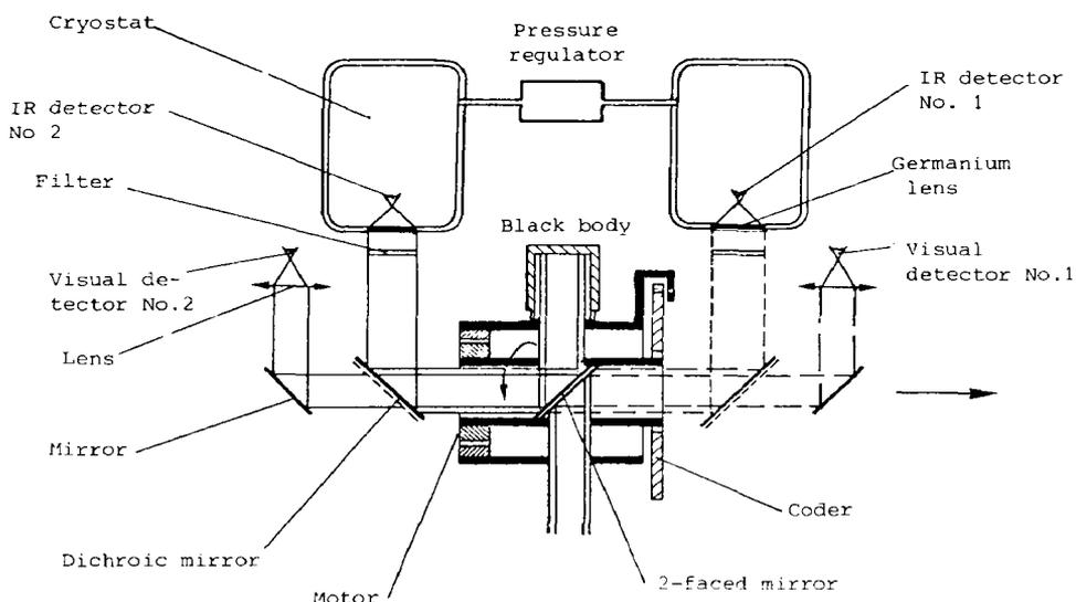
FIG. 9. — Scanning principle of Aries radiometer.
