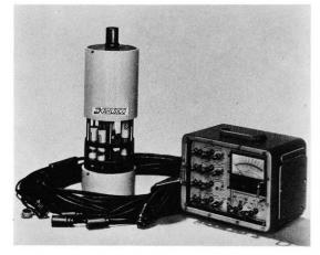
**HYDROLAB SYSTEM**, a modern and reliable in-situ measuring and monitoring system consisting of a control unit, cable and underwater sonde with sensors to measure various parameters including Temperature, Depth, Conductivity, Dissolved Oxygen, pH, Redox, Specific lon, etc. Accessory recorders and data loggers are available.
