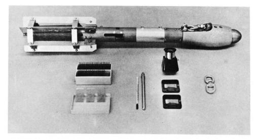
**KAHLSICO BATHYTHERMOGRAPH (BT)** is an efficient and reliable device which graphically records on a gold-plated glass slide both temperature and depth measurements as the BT is towed through the water at speeds up to 15 knots. It may be used to depths of 270 meters (900 ft). As illustrated, the equipment comes complete with all accessories, including a calibrated grid, viewer and thermometer, all packed in a special, compartmented storage case.
