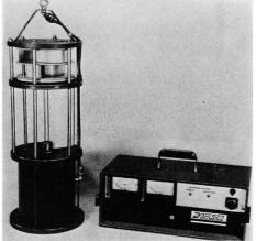
**REMOTE CURRENT METER**, uses a special Savonius rotor and coupled compass to provide accurate measurements of water speed and direction. Special design features make this the most reliable unit available. Accessory recorders and data loggers can be provided as well as temperature and depth measuring systems.
