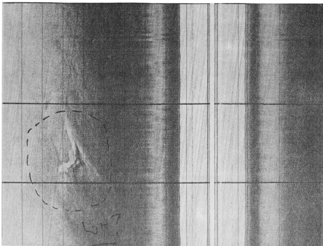
Bottom : Here the contact is in optimum relationship to the towfish, although the overall gain is slightly too high.
