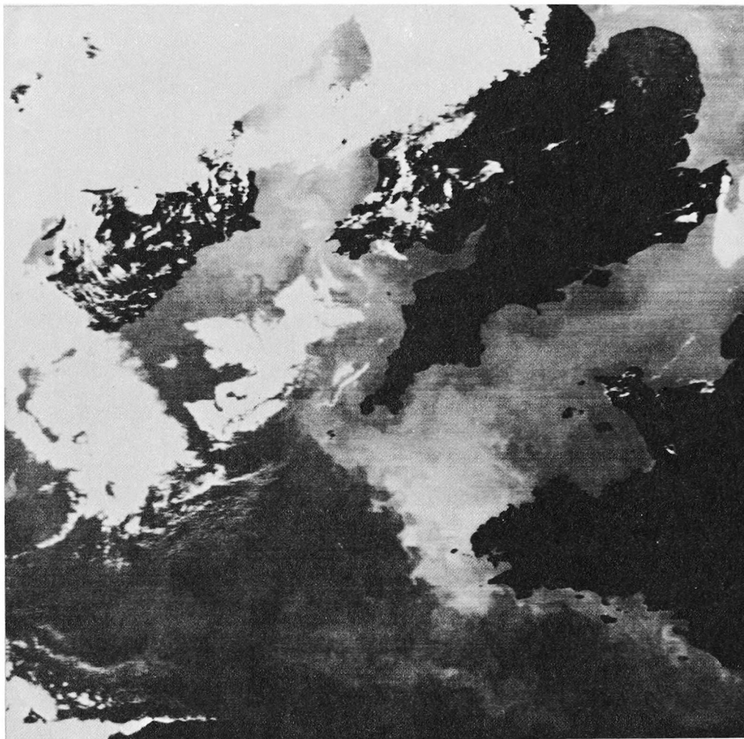
FIG. 2. — Infra-red image of the western approaches to the English Channel. Cloud covers the top left portion. The change in tone of the sea-surface across a line from Ushant to the Scillies denotes a strong 'oceanic front'.
