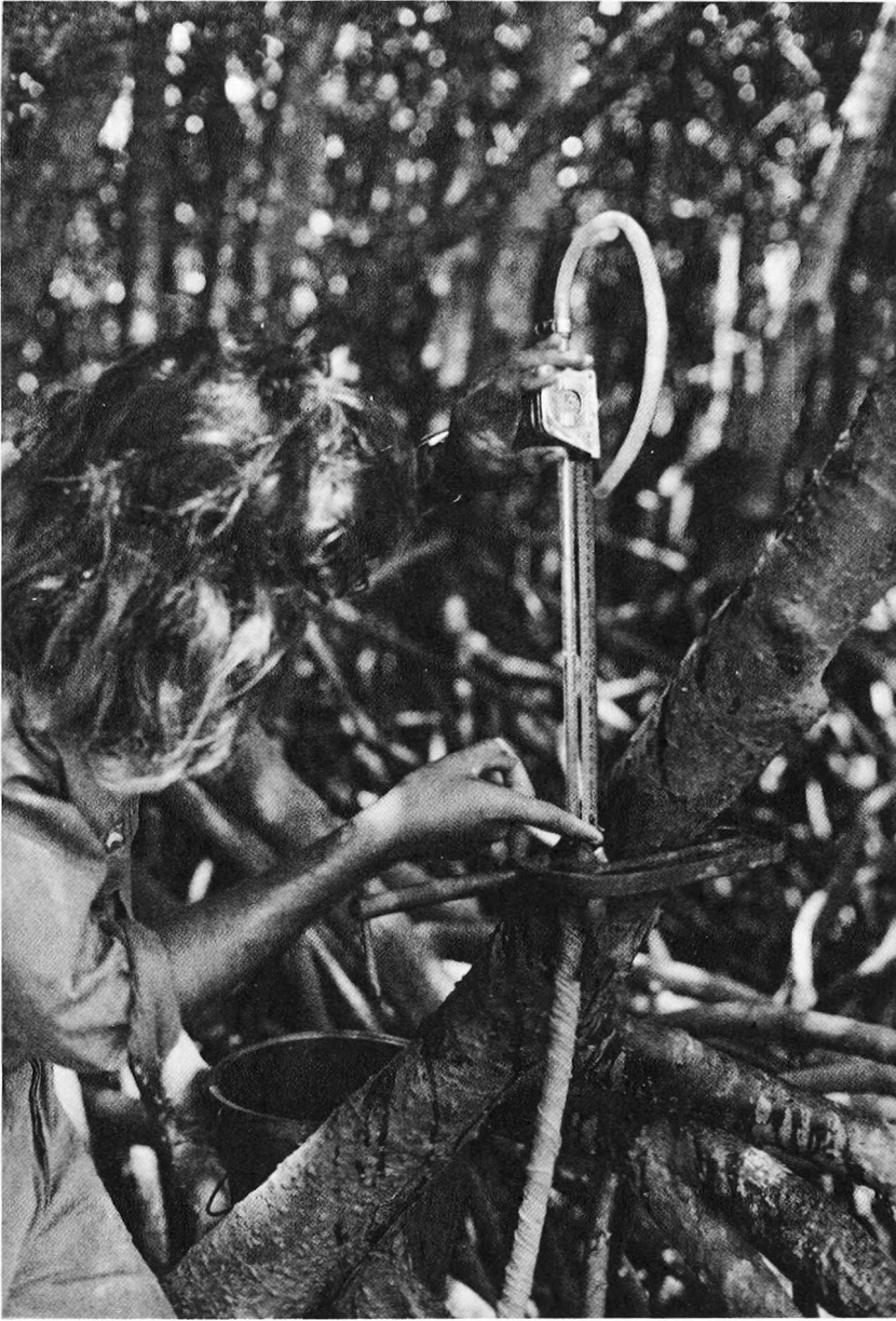
FIG. 2. — Taking the level with a measuring tape. Note the G-clamp, the length of plastic tubing and the wetted bandage on the main hose.
