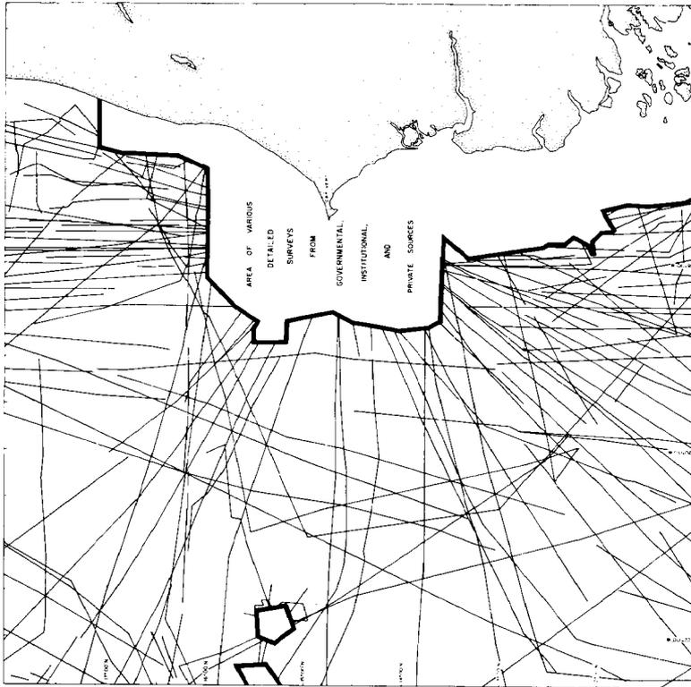
FIG. 1B. — Map of survey area showing all the additional lines of bathymetry which were compiled into map 839A. All these lines were either from scientific research vessels of various nations or were judged to have a high quality of positioning which would permit them to be integrated with the *Baffin* data. Sources are all detailed in the tables of RUFFMAN *et al.* (1977 a, 1977 b).
