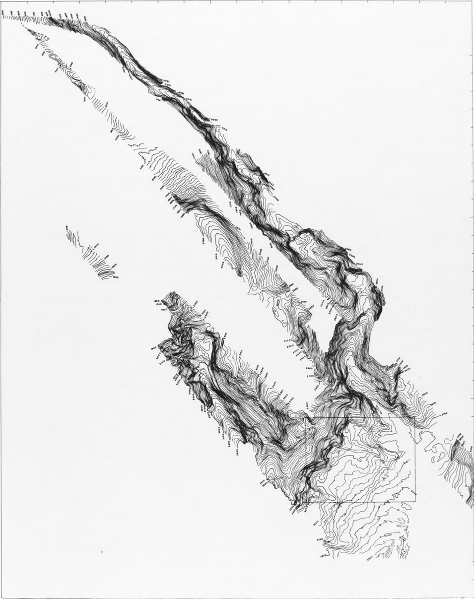
FIG. 27. — Bathymetric map assembled from Sea Beam plots and Decca navigation. Test Area 1 is outlined. Frame marks spaced at one minute of latitude or longitude, contour interval 20 m.
