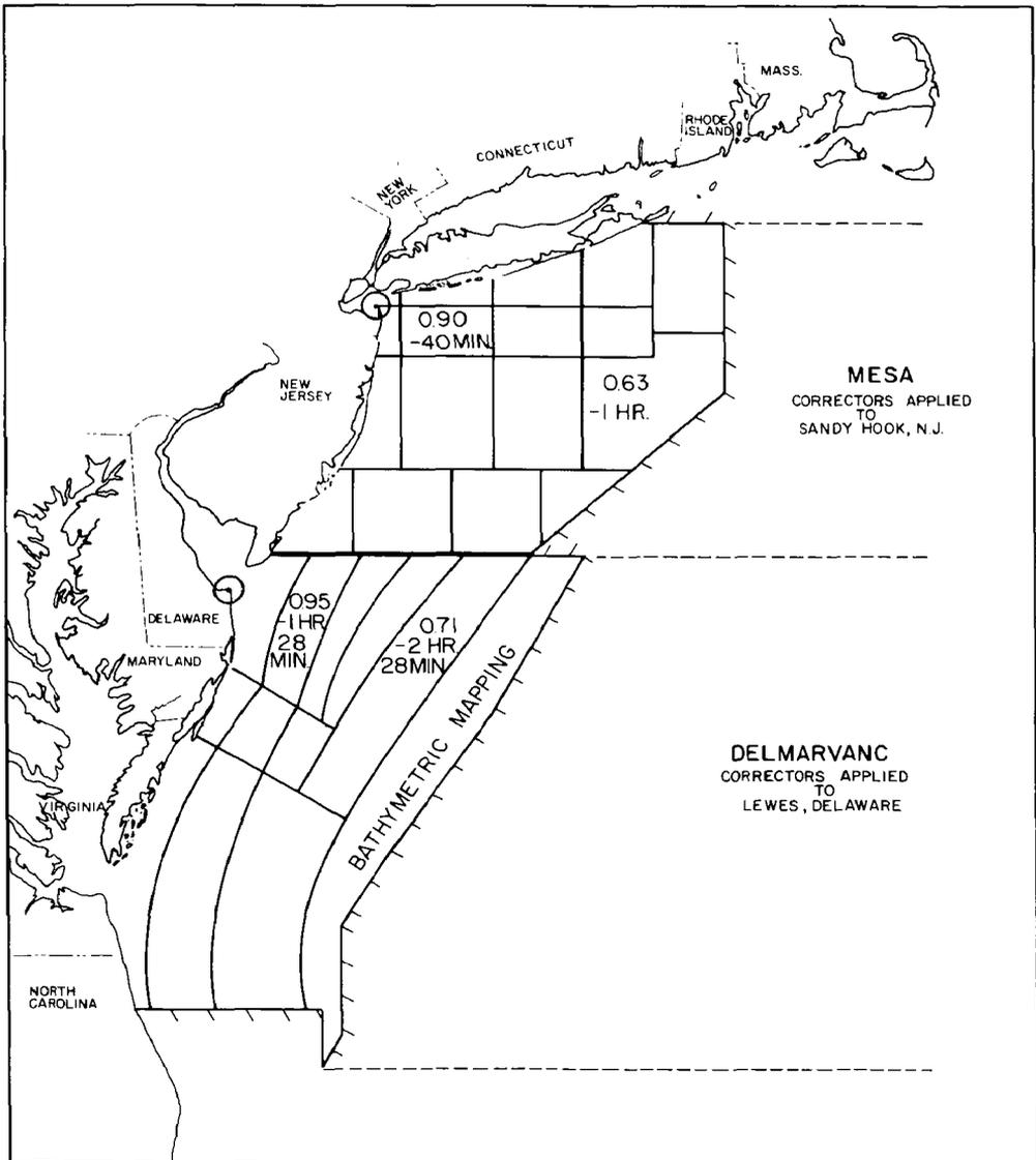
FIG. 1. — Preliminary tidal zoning where the upper number is the height ratio and the lower number the time correction.
