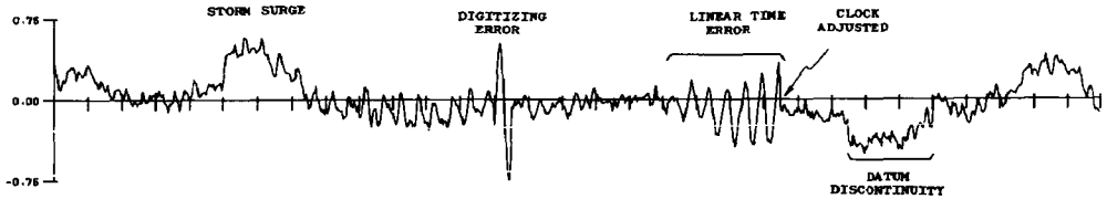
FIG. 2. — Typical features, due to various error effects or other influences, which can be identified in a residual time series.
