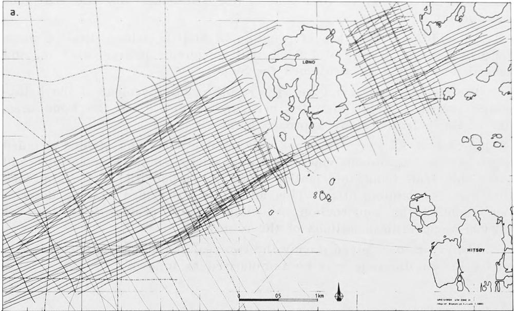
FIG. 7a. — Detailed nearshore route survey lines run during mapping Steps 1 and 2 in 1977 and previously, in the Løno area.
