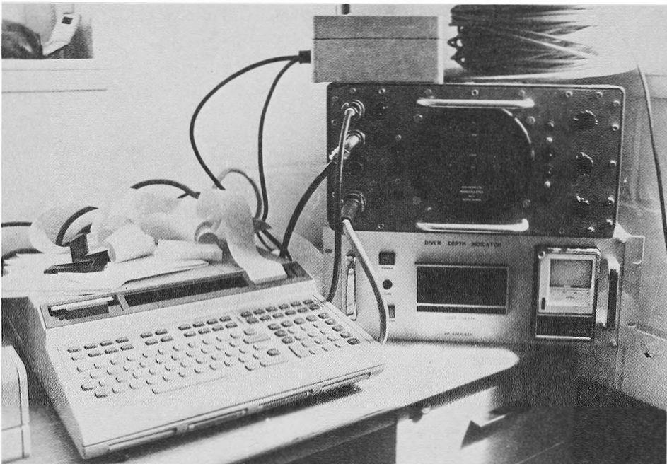
FIG. 6. - Sonardyne Rangemaster 'MF' Console with four slant ranges shown in circular display panel. The Diver Depth Indicator used to monitor the transducer depth is also fed directly into the HP9825S.
