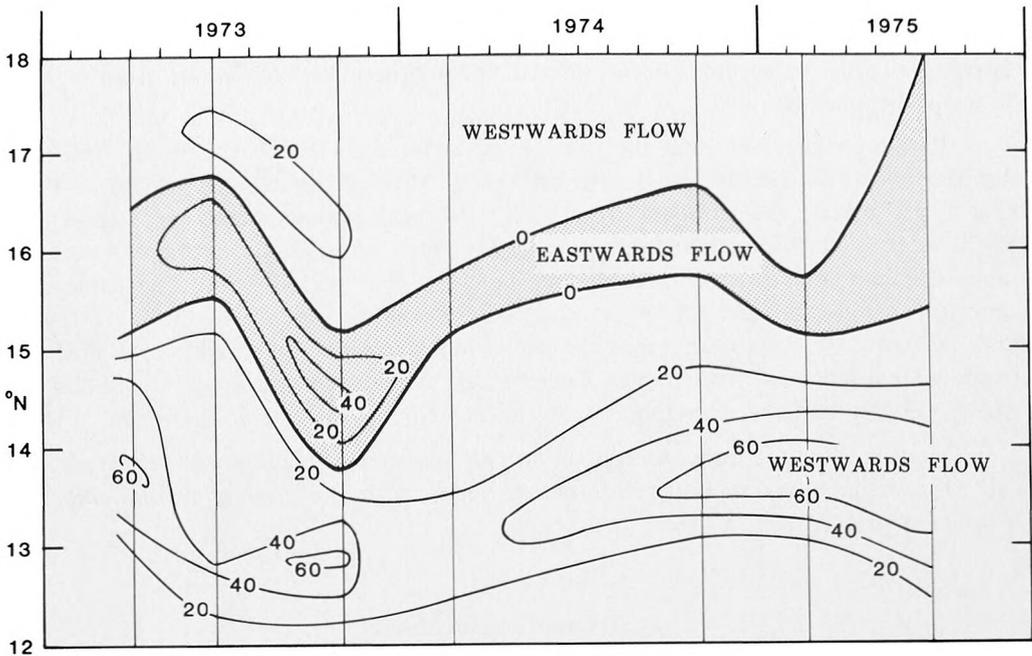
FIG. 10. - Metachronic map of surface velocities (cm/sec) along 67°W (calculated geostrophically relative to 1 600 db).
