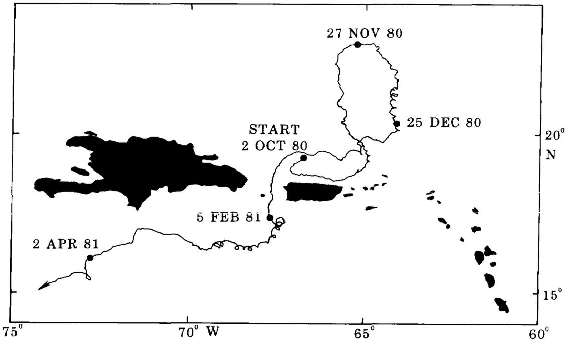
FIG. 7. — Track of a buoy launched off the north coast of Puerto Rico: 2 October 1980 - 15 April 1981. The buoy was tethered to a  $2\text{ m} \times 10\text{ m}$  window-shade drogue centred at a depth of 15 m. The drogue was lost on 13 April 1981, at which time the buoy's rate of drift increased appreciably.
