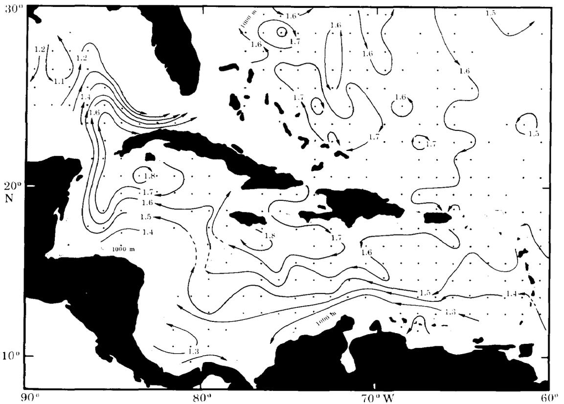
FIG. 3. — Surface flow patterns in January-March around the Greater and Lesser Antilles, deduced from the dynamic topography of the sea surface (0/1000 db in dynamic meters, averaged over one-degree squares). • Indicates data available. 1364 stations used.
