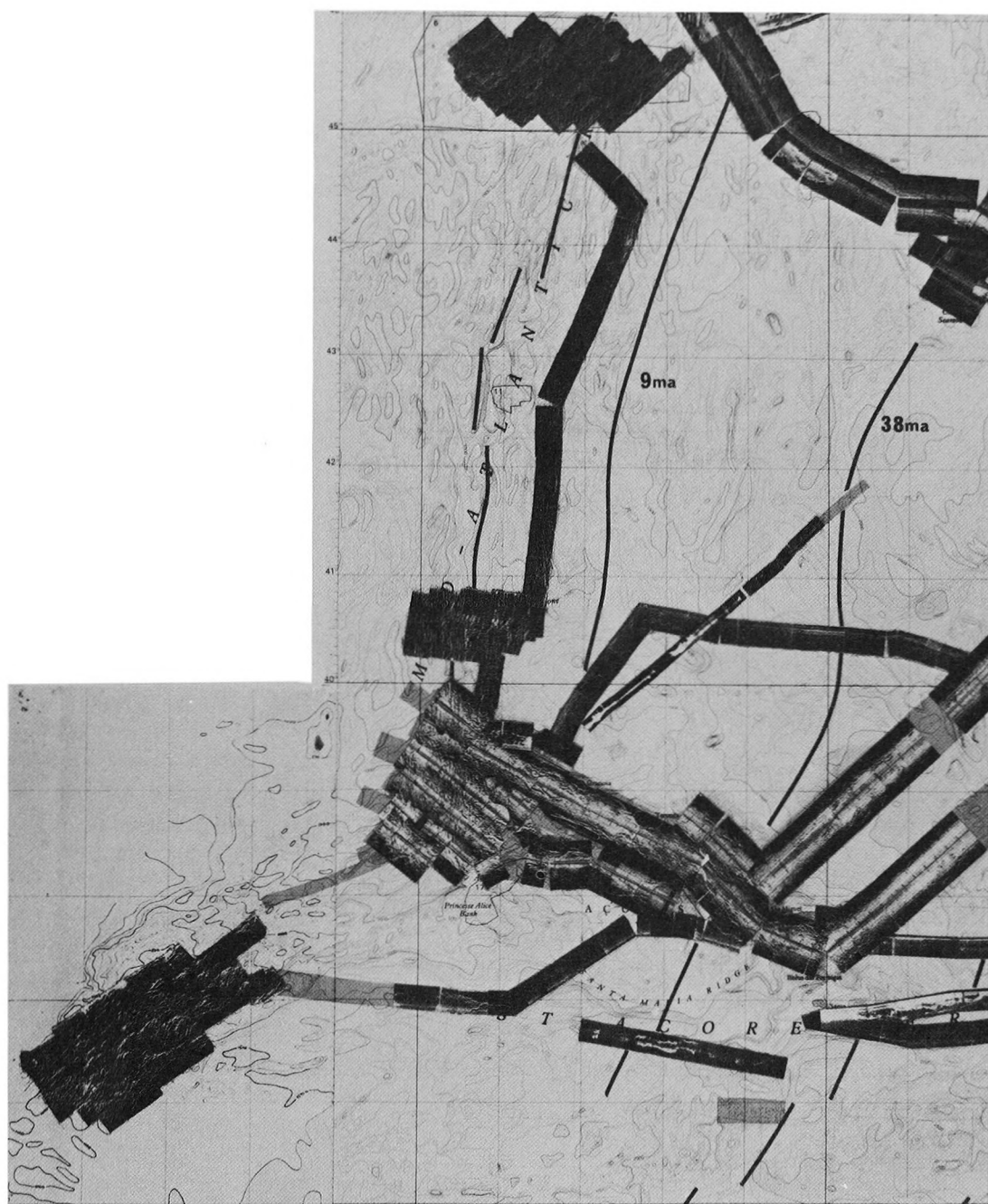
FIG. 18. — Sonographs mounted on part of the bathymetric chart Mid-Atlantic Ridge to South West Europe (LAUGHTON et al. , 1975), showing special studies of the Mid-Atlantic Ridge axis at 45° N, the Kurchatov Fracture Zone, the Azores triple junction, and the FAMOUS area, and of the Azores platform. The islands of the Azores in the survey area are black. Heavy black lines give the 0.9, and 38 Ma isochrons.
