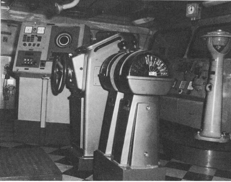
FIG. 3. — View of the bridge showing the auto-pilot, engine controls, compass pelorus, etc.
