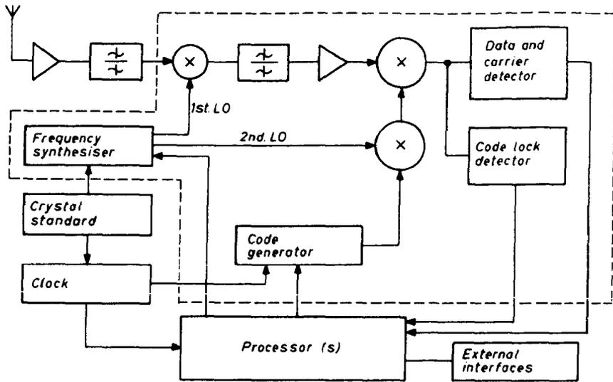
FIG. 3. — Typical Navstar receiver.
