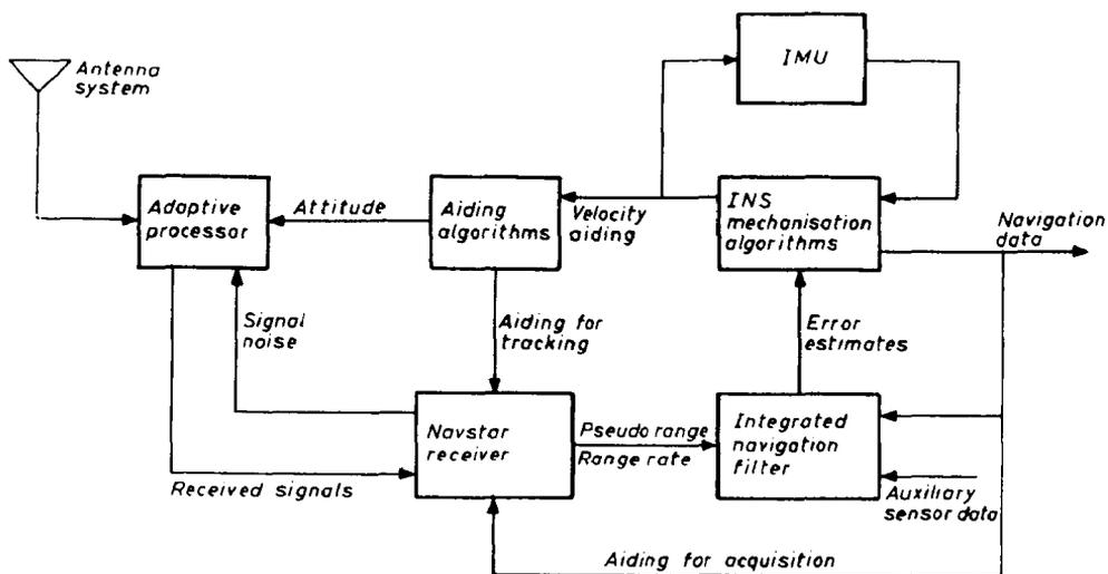
FIG. 4. — Integrated navigation system (Navstar/INS).
