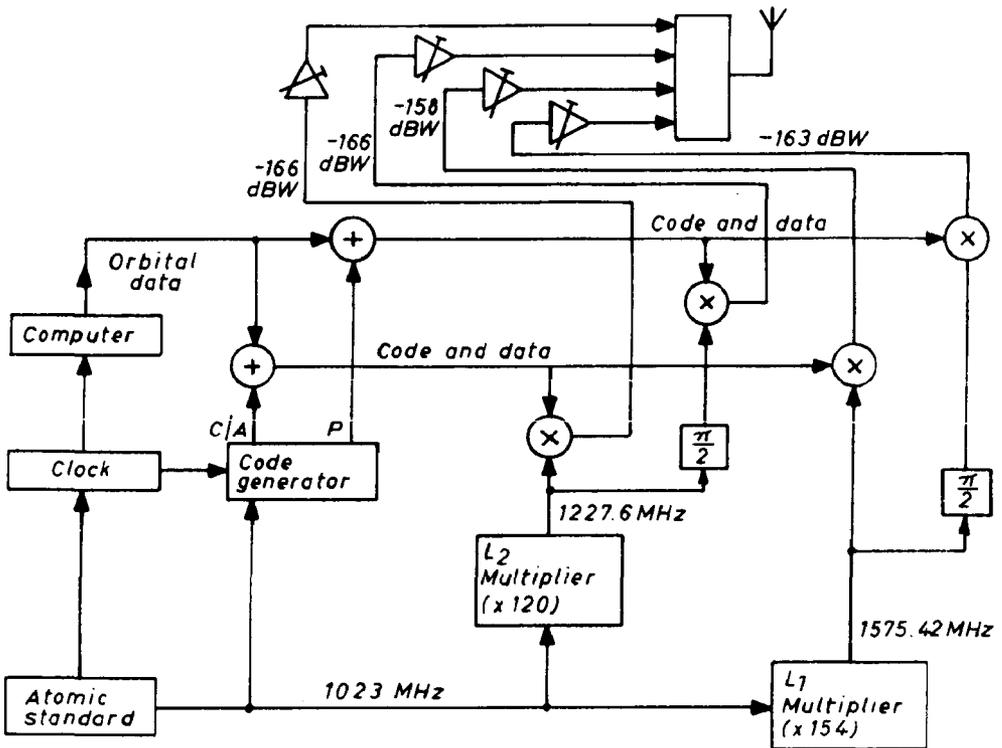
FIG. 1. — Schematic satellite signal generation.
